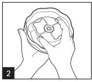
Squeeze locking tabs and remove motor housing from lid.
