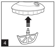
Insert mixing paddle into motor housing.
