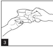
Wipe motor housing with a damp cloth. Do not immerse in water or other liquid.
