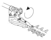
Press the cutting unit against the hedge or some other firm surface until the required angle is set.
