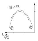
**CAUTION!** If the blades move while the engine is idling the T screw should be turned anti-clockwise until they stop.
