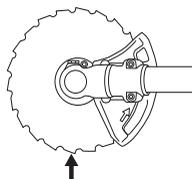
When loosening and tightening the saw blade nut, there is a risk of injury from the teeth of the saw blade. You should therefore always ensure that your hand is shielded by the blade guard when doing this. Always use a socket spanner with a shaft that is long enough to allow this. The arrow in the diagram shows the area where you should
