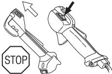
Start the engine and make sure the engine stops when you move the stop switch to the stop setting.
