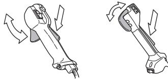
See instructions under the heading Start. Start the machine and apply full throttle. Release the throttle and check that the cutting attachment stops and remains at a standstill. If the cutting attachment rotates with the throttle in the idle position then the carburettor idle setting must
