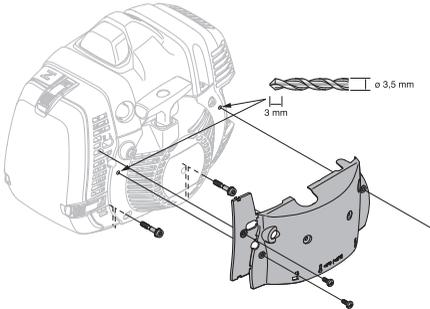
**IMPORTANT!** The machine **MUST** be returned to its standard design at temperatures warmer than 5°C (41°F). Otherwise there is a risk of overheating resulting in serious engine damage.
