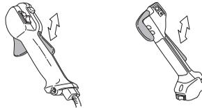
Check that the throttle trigger and throttle lockout move freely and that the return springs work properly.
