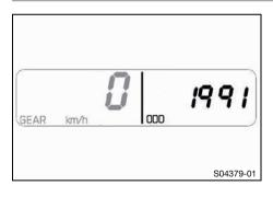
Press the + or - button repeatedly until ODO is shown on the combination instrument.
