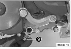
Mount and tighten screw plug with the O-ring. Guideline
