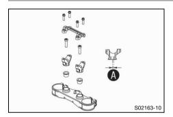
The holes on the handlebar support are placed at a distance of  $\mathbf{A}$  from the center.
