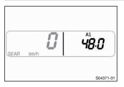
Press the + or - button repeatedly until A1 is shown on the combination instrument.
