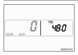
Press the + or - button repeatedly until TR2 is shown on the combination instrument.
