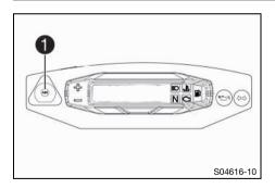
The ABS button **1** is fitted next to the combination instrument on the left.
