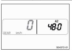
Press the + or - button repeatedly until A2 is shown on the combination instrument.
