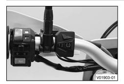
The combination switch is fitted on the left side of the handlebar. The combination switch is fitted on the left side of the handlebar.
