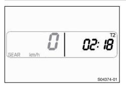
Press the + or - button repeatedly until T2 is shown on the combination instrument.
