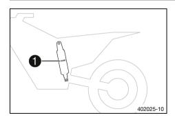
The shock absorber article number **1** is on the left side of the shock absorber.
