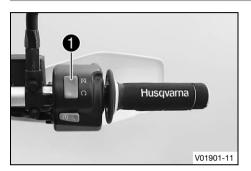
The emergency OFF switch **1** is fitted on the right side of the handlebar.
