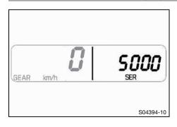
Press the + or - button repeatedly until SER is shown on the combination instrument.
