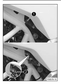
Clean quick release coupling 1 thoroughly with compressed air.
