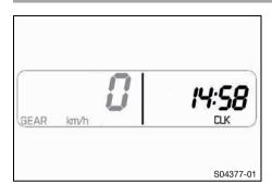
Press the + or - button repeatedly until CLK is shown on the combination instrument.
