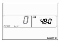
Press the + or - button repeatedly until TR1 is shown on the combination instrument.
