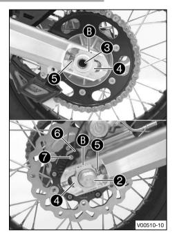
Clean and grease the thread of the wheel spindle and nut 2.
