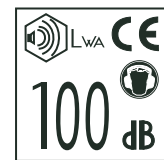
Noise emissions to the surroundings in accordance with the European Union's directive. The machine's emission is stated in the chapter TECHNICAL DATA and on the decals. Only machines for European market
