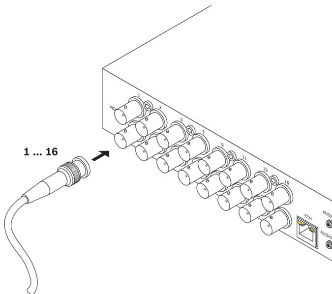
You can connect a maximum of 16 video sources to the VIDEOJET multi 4000 encoder. Any cameras and other video sources that produce a standard PAL or NTSC signal are suitable.
