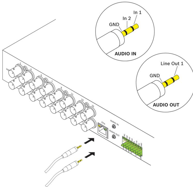
The unit has two audio ports for audio line signals. The audio signals are transmitted two-way and in sync with the video signals. The following specifications should be complied with in all cases.
