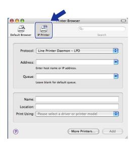
(Mac  $OS^{\$}$  X 10.2.4 to 10.3.x) Enter the IP address of the printer into the **Printer Address** box. (Mac  $OS^{\$}$  X 10.4) Enter the IP address of the printer into the **Address** box.
