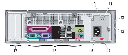
**NOTE:** The voltage selector switch is available only on non-EPA power supplies.
