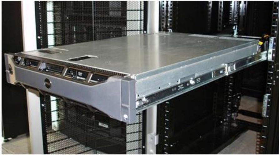
Figure 14. R710 Mounted in B1 Sliding Rails
