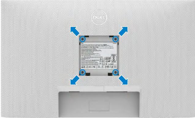
**NOTE:** Use M4 x 11 mm screws to secure the wall-mounting kit to the monitor.
