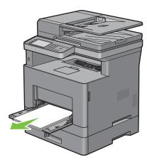
**2** Grasp both sides of the MPF, and then pull the MPF from the printer.
