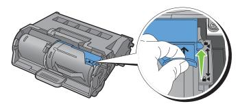
**5** Grasp the handle on the toner cartridge, and then pull it out of the old drum cartridge.
