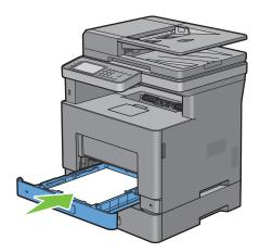
**10** Insert the MPF into the printer, push until it stops, and close the MPF.
