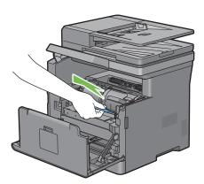
**3** Hold both sides of the drum cartridge with your hands, and then pull it out completely.
