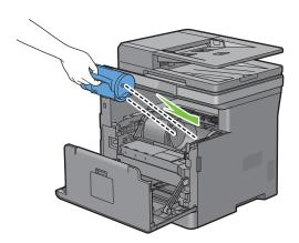
Grasp the toner cartridge lock lever, and then pull it down until it stops.
