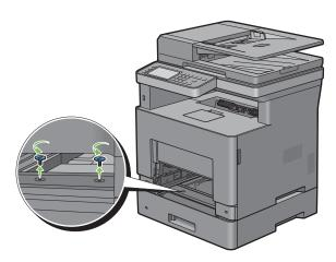
7 Gently lift the printer off the optional 550-sheet feeder, and place it on a level surface.
