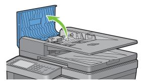
Lift the release lever 90 degrees and remove the jammed document by carefully pulling it to the right.
