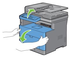
**2** Grasp the handle on the front of the drum cartridge, and then pull it out halfway with one hand.
