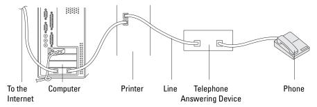
If you want to use your computer modem for faxing or for a dial-up Internet connection, connect the computer modem directly to the rear of your printer with the TAD as shown above.
