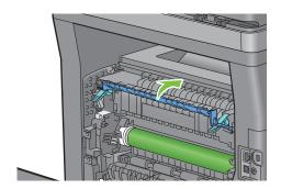
7 Press down the levers on both sides of the fusing unit.
