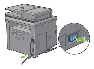
**NOTE**: The data in the memory are cleared when the printer is turned off.
