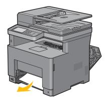
**7** Insert trayl into the printer, and push until it stops.
