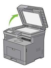
2 Place the document facing down on the document glass and align it with the registration guide on the top left corner of the glass.
