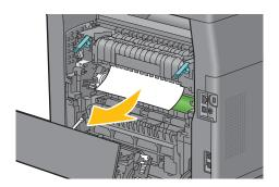
4 If the document is jammed above the fusing unit, raise the tab of the inner part, and turn it to open.
