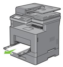
**2** Grasp both sides of the MPF, and then pull the MPF from the printer.
