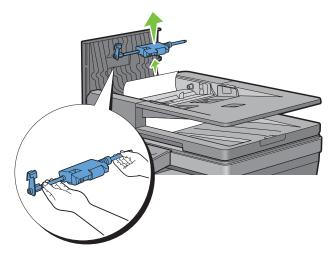
Insert the DADF feed roller assembly and press down the release lever.
