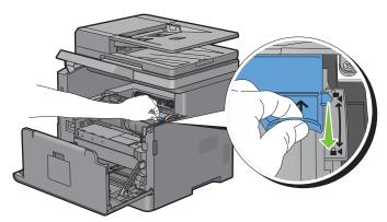
Close the front cover, and put back the operator panel to the original position.
