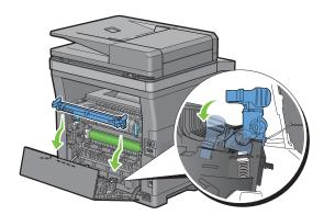
4 Make sure that the arrow marks on the transfer unit and the printer face each other, and then press the two tabs on transfer unit inward to lock.
