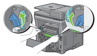
**4** Grasp the grips on both sides of the fusing unit, and then pull out the unit.
