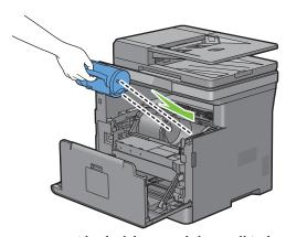
7 Grasp the toner cartridge lock lever, and then pull it down until it stops.
