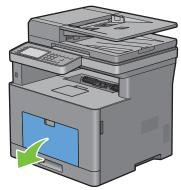
**3** Grasp both sides of the MPF, and then pull the MPF from the printer.
