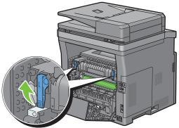
**3** Slide the envelope switches on the both sides of the fusing unit to the [ position.
