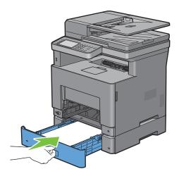
**9** Insert trayl into the printer, and push until it stops.
