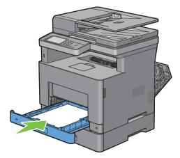
11 Insert the MPF into the printer, push until it stops, and close the MPF.
