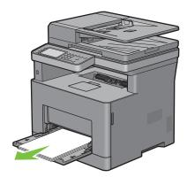
**2** Grasp both sides of the MPF, and then pull the MPF from the printer.
