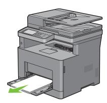
**2** Grasp both sides of the MPF, and then pull it out of the printer.
