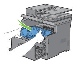
**3** Grasp the handle on the front of the drum cartridge, and then push and install the drum cartridge until it stops.
