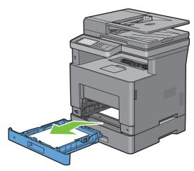
**5** Pull the optional 550-sheet feeder from the printer about 200 mm.
