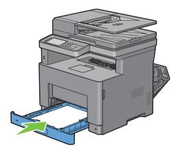
**8** Insert the MPF into the printer, push until it stops, and close the MPF.
