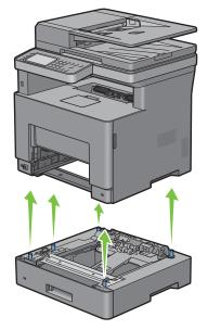
**8** Insert trayl into the printer, and push until it stops.
