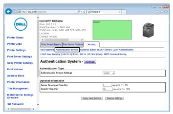
2 From the Authentication System Settings drop-down menu under Authentication Type, select LDAP as the authentication method, and then click Apply New Settings.
