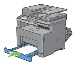
8 Insert the MPF into the printer.
