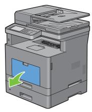
**3** Grasp both sides of the MPF, and then pull the MPF from the printer.
