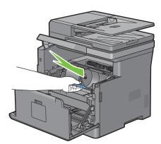
To remove the toner cartridge from the old drum cartridge, grasp the toner cartridge lock lever, and then raise it upward to unlock.
