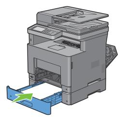
**10** Insert trayl into the printer, and push until it stops.
