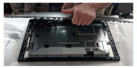
Remove the tape which fixed USB FFC cable and USB wire on panel.
