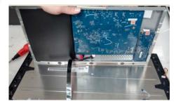
S17 Unlock 11 screws on Middle frame
