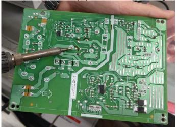
S26-4 Lift the bulk cap. up and away from the PCB
