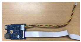
S10 Remove Sensor BD wire from I/F BD and Sensor BD
