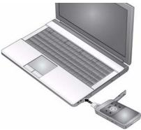
NOTE: It may be convenient to use a USB extension cable to connect the camera to the computer.
