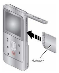
**IMPORTANT:** When you turn on the camera, it checks to see if a card is inserted. If so, new pictures/videos are stored on the card. If no card is inserted, new pictures/videos are stored in the camera internal memory. If pictures/videos are detected in internal memory and a card is inserted, the camera prompts you to move the pictures to the card (and erase those in internal memory).
