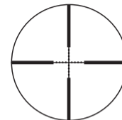
Fig. 3-3 Milliradian Dot Reticle
