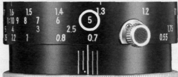
The reproduction ratio is, numerically, the relationship between the image size (to be recorded on the film) and the actual subject size. For example, if the image on the focusing screen is one-fifth the actual subject size, the reproduction ratio is 1:5.
