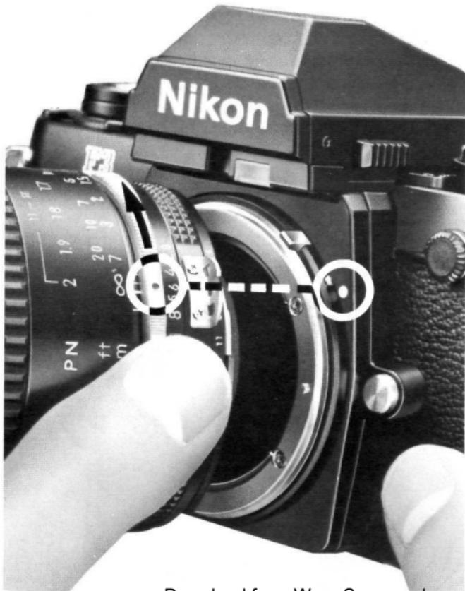
Grasp the lens by its mounting ring. Position the lens in the camera's bayonet mount, lining up the aperture index on the lens with the lens mounting index on the camera, and twist the lens counterclockwise until it clicks into place.
