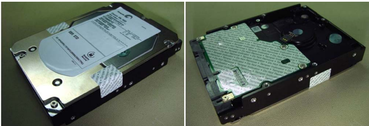
Figure 10. Example of FIPS tamper evidence labels.
