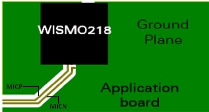
Figure 24. Single-Ended Audio Connection
