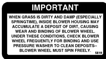
Top of Blower Housing (5819)
