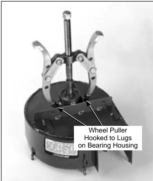
Pressing Blower Wheel Out of Housing
