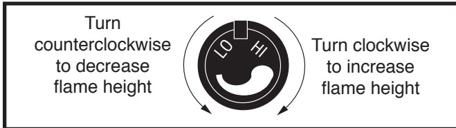
Fig. 56 Flame adjustment knob for Honeywell valve.
