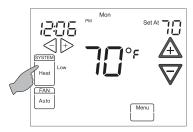
Touch the **SYSTEM** key to select the thermostat operating mode desired. When the system is calling for first stage heat or cool, "**Low**" will display on the touchscreen. When second stage is required, the display will show "**High**". The setpoint temperature can be changed by touching the  $\triangle$  or  $\nabla$  keys.
