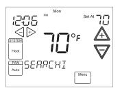
During power up, the thermostat will scroll the word "SEARCHING" in the message area, indicating that the system is looking for components (Air Handler, Furnace, Heat Pump, Air Conditioner) on the Climate Talk network. Once the components are identified the message display will indicate the components found. Confirmation will be given in the message area that the equipment has been found with the message (equipment) FOUND.
