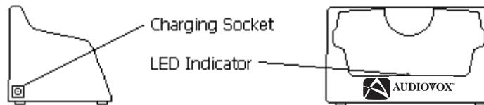
**Important:** The charging stand in your kit is intended for use with the RBP-214 batteries included in the kit. Do not attempt to recharge any other batteries with the charging stand.
