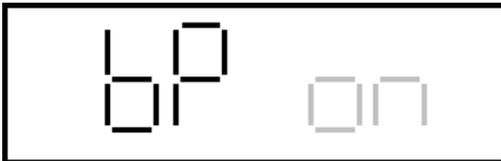
The display will show "bpxxx" indicating the status of the button conformation beeps, on or off. Pressing the up or down buttons, within 5 seconds will turn the button conformation beeps on or off. When the beep tones are on, pressing the up, down or lock buttons will be confirmed by a beep tone. A double beep tone will sound whenever the unit is turned on or off. When the conformation beeps are off all beep tones will be eliminated.
