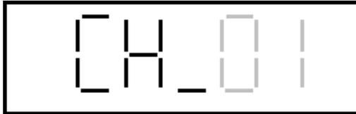
The channel number will flash on the display, beginning the function selection sequence again. If the conformation beeps are on, a double tone will be heard.
