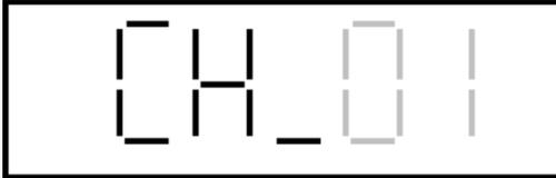
The channel number will flash on the display, indicated by "CH\_xx." Pressing the up or down buttons, momentarily, within five seconds will increment or decrement through the 14 channels one at a time.
