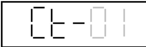
The CTCSS privacy code will flash on the display indicated by "Ct-xx." Pressing the up or down buttons, within 5 seconds will change through the 38 CTCSS privacy codes one at a time.
