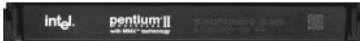
Intel Pentium II Processor in a SEC Cartridge (233-333MHz 512KB/256KB/0KB L2 Cache)
