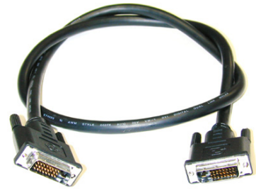
Image 3-17 DVI-DVI data cable of 0,9 meter (R9851211).
