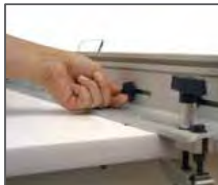
Adjusting the sub-fences is easy. No tools required!
