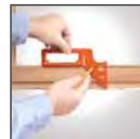
Accurately mark 3/16" reveals around window and door jamps
