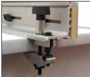
Close-up photo of the cantilever clamps. Large T-knobs are easy on the hands.
