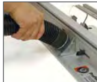
Built-in dust collection for 2-1/2" shop vac hose.
