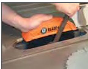
Place Blade-Loc over your blade and tighten.
