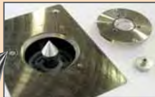
Centering cone installed, ready to center guide bushing adapter to router.
