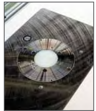
Zero clearance insert installed in a ProLift. Use when routing very small stock.
