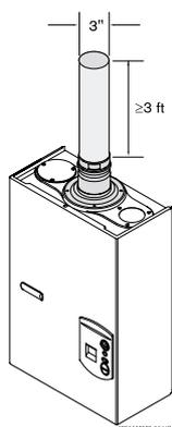
The use of a 90 degree elbow is equivalent to 2½ ft in vent length.
