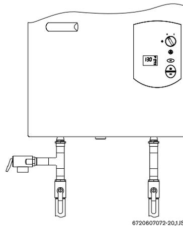
Fig. 25 Plumbing Connections and Pressure Relief Valve
