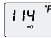
Fig. 35 Locked condition
