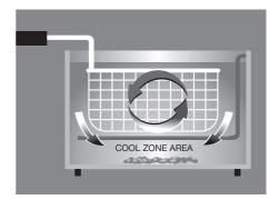
The submerged heating element system on the deep fryer allows oil to be heated more effectively, and respond quickly to oil temperature changes.
