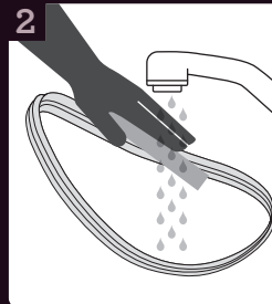
2 Wash silicone rubber gasket.
