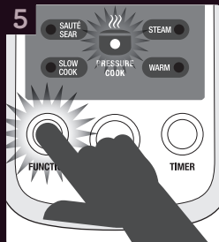
5 Press FUNCTION button until the Pressure Cook indicator light flashes.
