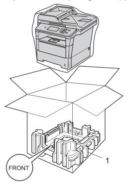
5 Put the packing material (2) marked "RIGHT" on the right of the machine. Put the packing material (3) marked "LEFT" on the left of the machine. Put the AC power cord and printed materials in the original carton as shown in the illustration.
