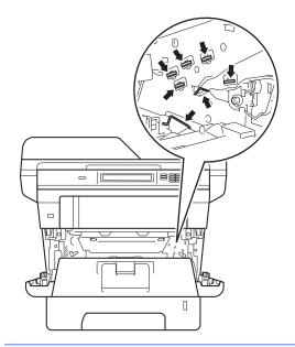
Clean the corona wire inside the drum unit by gently sliding the green tab from left to right and right to left several times.
