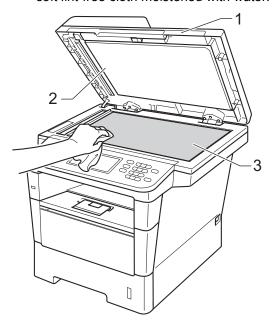
In the ADF unit, clean the white bar (1) and the glass strip (2) underneath it with a soft lint-free cloth moistened with water.
