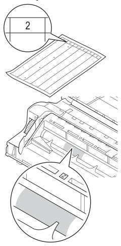
Turn the drum unit gear toward you by hand while checking the surface of the suspected area.
