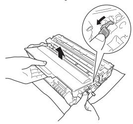
Turn the drum unit as shown in the illustration. Make sure that the drum unit gear (1) is on the left hand side.
