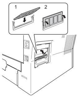
6 Put the plastic SO-DIMM cover (1) back on.
