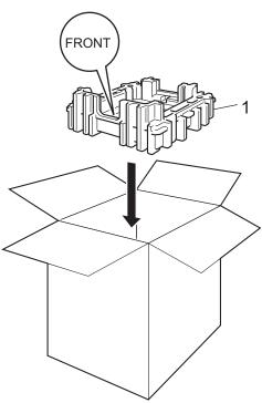
Wrap the machine in a plastic bag, then put it on the bottom packing material (1).
