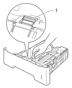
Wipe the two pick-up rollers (1) inside of the machine to remove dust.
