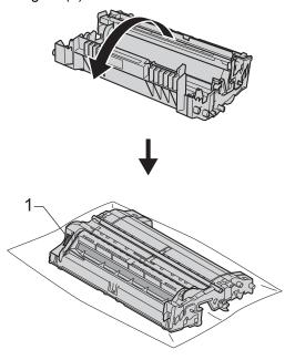
Use the numbered markers next to the drum roller to find the mark. For example, a dot in column 2 on the check sheet would mean that there is a mark in the "2" region of the drum.
