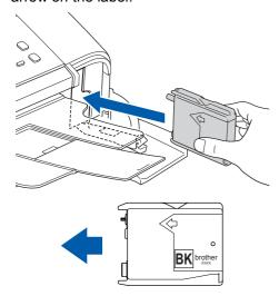
Lift the lock release lever and gently push until it clicks, and then close the ink cartridge cover.
