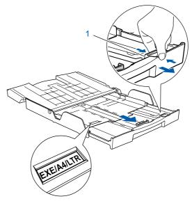
Press and slide the paper side guides (1) and paper length guide (2) to fit the paper size.
