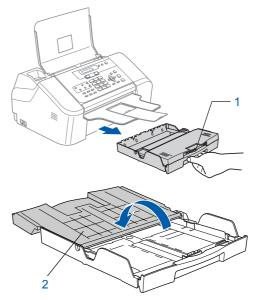
If you are using Letter, A4 or Legal size paper, press and hold the universal guide release button (1) as you slide out the front of the paper tray to match the paper size you are using.
