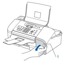
Pull the lock release lever down and remove the yellow protective part (1).
