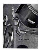
When the camera is not in use. rotate the LOCKING RING clockwise until a red mark appears. When this is done, the EXPOSURE LEVER is locked to prevent accidental tripping. To unlock, rotate the LOCKING RING back until the red mark is concealed. With the EXPOSURE LEVER pressed down, the LOCKING RING can be rotated further in the same direction (still concealing the red mark). This will lock the lever in position for continuous taking.
