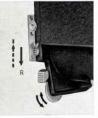
TROL to "R". With the control pointed at "R" and the EXPOSURE LEVER pressed down, continuous running shots can be taken. When the control is placed at "1", single frame picture can be taken by pushing up the EXPOSURE LEVER. In both cases, shutter can not be operated if the EXPOSURE LEVER SAFETY LOCK is locked.
