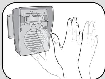
Test PIR Motion Sensor by waving hand in front of sensor. Test light should flash after several seconds.
