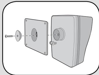
Connect PIR Motion Sensor box to mounting plate with silver screw. Tighten screw until PIR Motion Sensor stays in place when repositioned.
