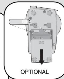
Plug in Base Station. Adhere rubber pads to bottom. 4 AA Alkaline batteries (not provided) are optional in case of power failures.
