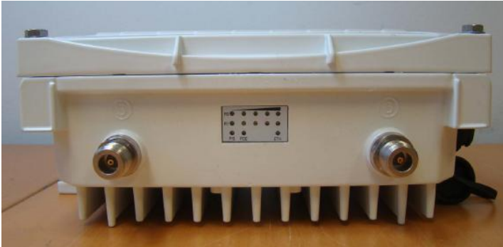
Figure 20 - Aruba AP-175 Tel placement back view
