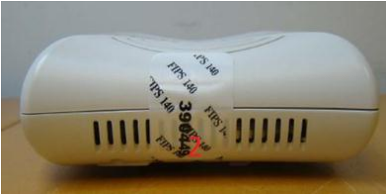
Figure 16 - Aruba AP-105 Tel placement left view
