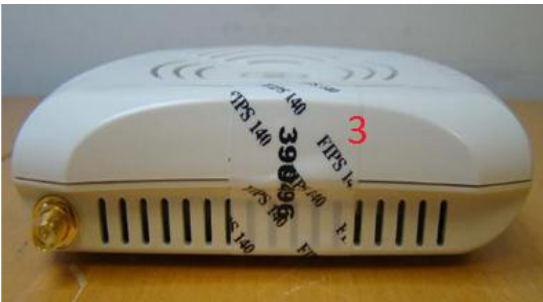
Figure 6 - Aruba AP-92 Tel placement left view
