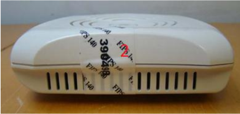
Figure 11 - Aruba AP-93 Tel placement left view
