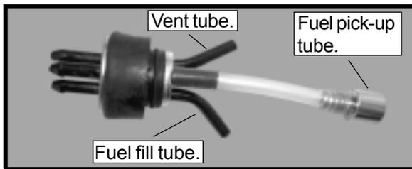
Carefully use a lighter or heat gun to permanently set the angle of the vent tube.
