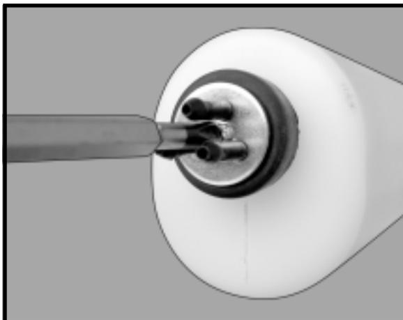
Attach the silicone fuel and pressure pipes to the tank. The lower pipe is the 'feed' and the upper two the 'pressure and fill'. The fill pipe is the next pipe.
