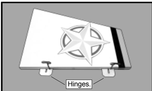
□ 3) Slide the rudder on the vertical fin until there is only a slight gap. The hinge is now centered on the fuselage panel and rudder. Remove the T-pins and snug the rudder against the fuselage panel. A gap of 1/64" or less should be maintained between the vertical fin panel and rudder.
