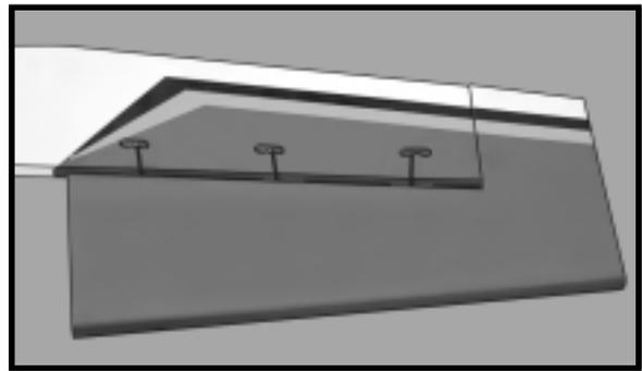
□ 4) Deflect the elevator and completely saturate each hinge with thin C/A glue. The elevators front surface should lightly contact the horizontal stabilizer during this procedure. Ideally, when the hinges are glued in place, a 1/64" gap or less will be maintained throughout the length of the elevator to the horizontal stabilizer panel hinge line.
