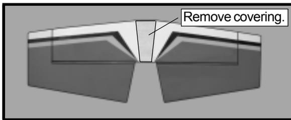
**!** *When cutting through the covering to remove it, cut with only enough pressure to only cut through the covering itself. Cutting into the balsa structure may weaken it.*
