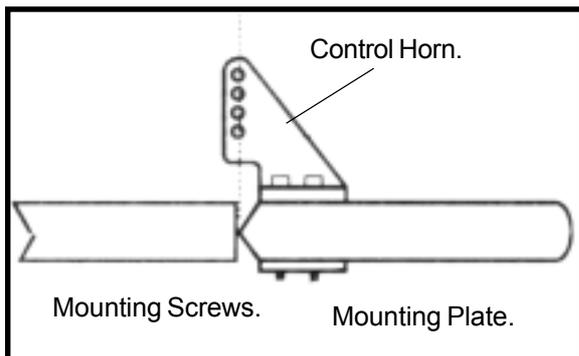
□ 3) Using a 1.5mm drill bit and the control horns as a guide, drill the mounting holes through the elevator halves.
