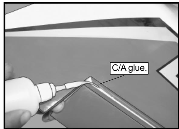
□ 5) Turn the wing panel over and deflect the aileron in the opposite direction from the opposite side. Apply thin C/A glue to each hinge, making sure that the C/A penetrates into both the aileron and wing panel.
