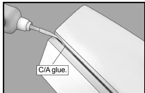
□ 6) Using C/A remover/debonder and a paper towel, remove any excess C/A glue that may have accumulated on the wing or in the aileron hinge area.
