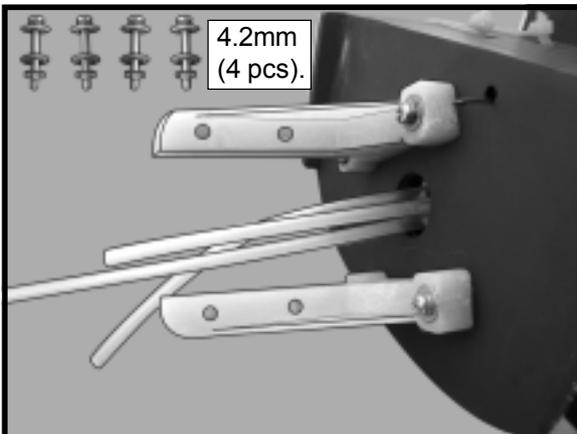
□ 5) Bolt the engine to the engine mount using the four machine screws. Double check that all the screws are tight before proceeding.
