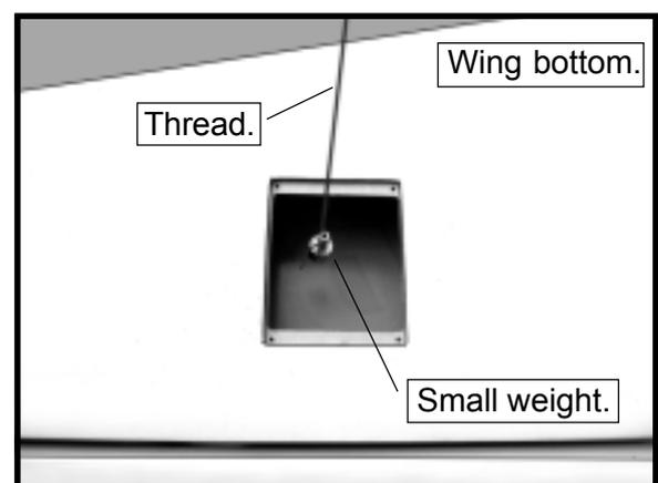
Attach the string to the servo lead and carefully thread it through the wing. Once you have threaded the lead through the wing, remove the string so it can be used for the other servo lead. Tape the servo lead to the wing to prevent it from falling back into the wing.
