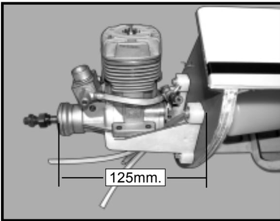
□ 2) Place your engine onto the engine mount. Adjust the engine is centered of the edges of the engine case.
