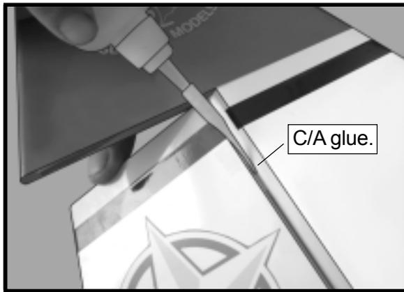
□ 5) Turn the vertical fin panel over and deflect the rudder in the opposite direction from the opposite side. Apply thin C/A glue to each hinge, making sure that the C/A penetrates into the rudder and fuselage panel.
