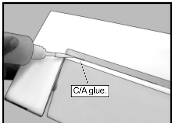
□ 6) Using C/A remover/debonder and a paper towel, remove any excess C/A glue that may have accumulated on the horizontal stabilizer or in the elevator hinge area.
