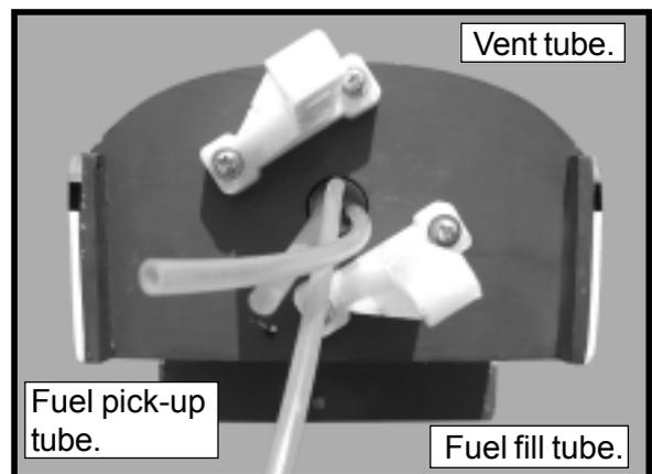
**!** *Blow through one of the lines to ensure the fuel lines have not become kinked inside the fuel tank compartment. Air should flow through easily.*
