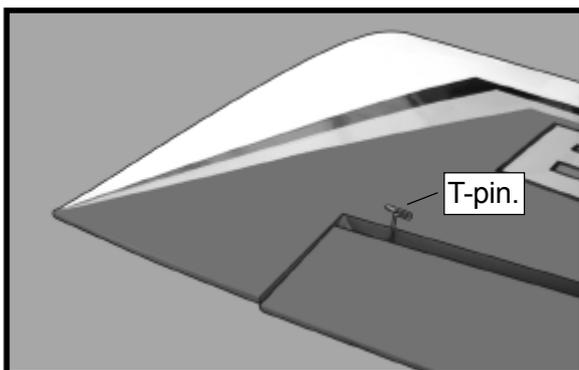
□ 4) Deflect the aileron and completely saturate each hinge with thin C/A glue. The aileron front surface should lightly contact the wing during this procedure. Ideally, when the hinges are glued in place, a 1/64" gap or less will be maintained throughout the length of the aileron to the wing panel hinge line.
