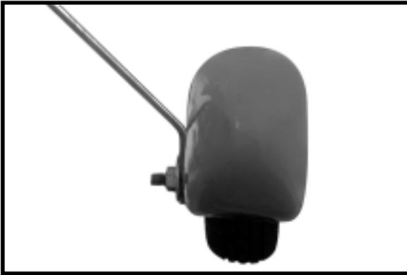
□ 4) A drop of C/A glue on the wheel collar screws will help keep them from coming loose during operation.
