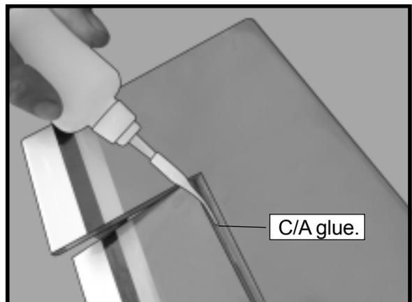
□ 5) Turn the horizontal stabilizer panel over and deflect the elevator in the opposite direction from the opposite side. Apply thin CA glue to each hinge, making sure that the C/A penetrates into both the elevator and horizontal stabilizer panel.
