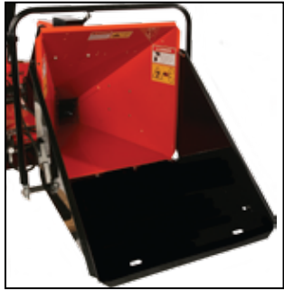
Fold down feed tray comes standard on the CH5540H (74554) Hydraulic PTO Chipper.
