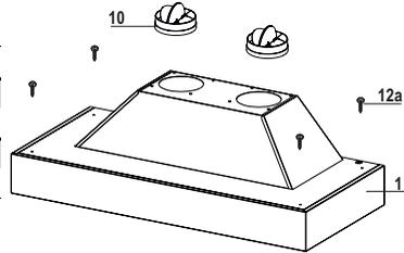
Hood support must be capable of supporting 40 lbs. (18,1 Kg) for 36" model or 55 lbs. (25 Kg) for 48" model.
