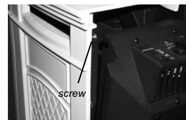
Lift Rear Panel off the 2 top screws
