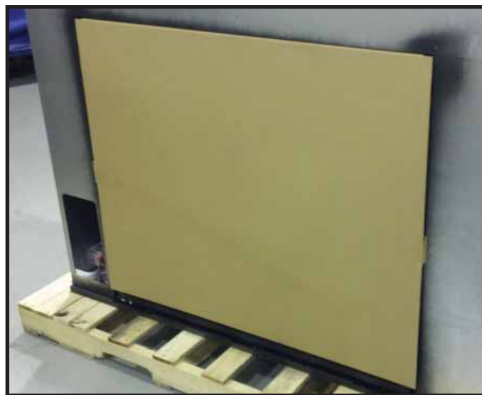
Figure 13.6. Splatter Guard Installation
