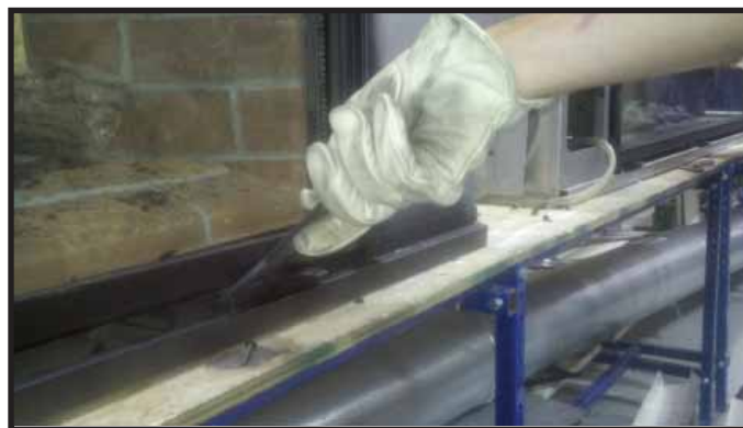
Figure 14.8. Inserting Glass Clip Tool
