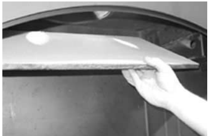
Figure 31B-Removing Baffle shown without ceramic blanket
