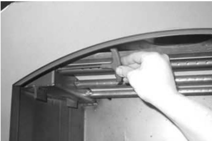
Figure 31A-Removing Manifold Tube
