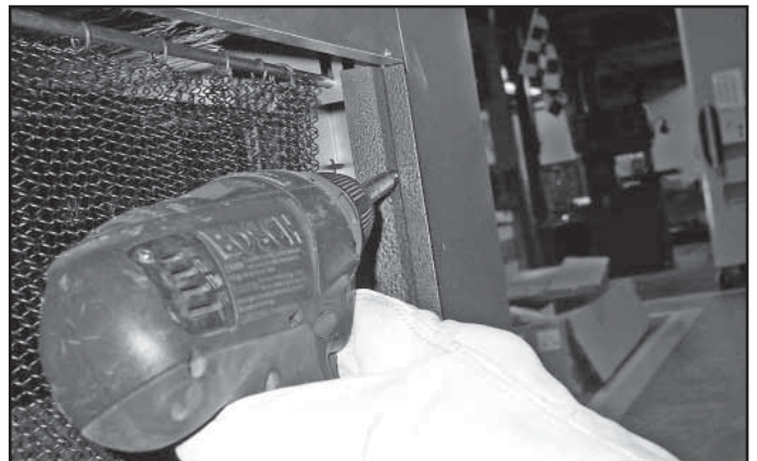
Figure 15.15 Install Refractory Shields
