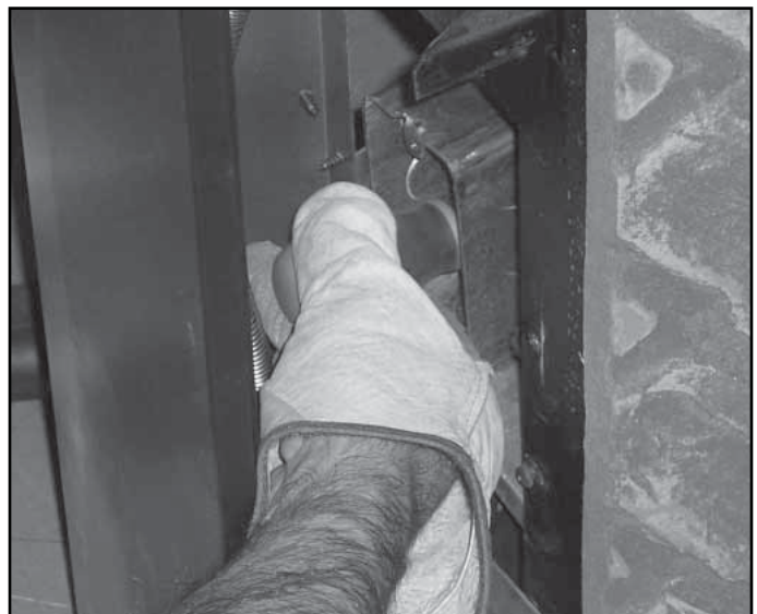
Figure 13.4 Remove Two Screws Holding Junction Box
