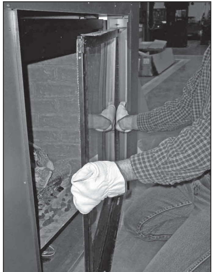
Figure 15.10 Remove Left Side of Glass Frame First
